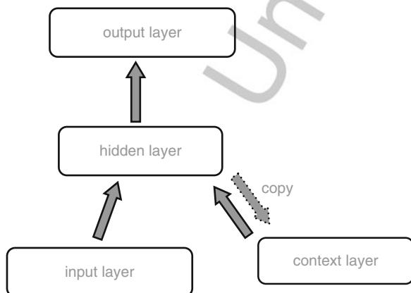
**Connectionism. Fig. 4** The Simple Recurrent Network (Elman 1990)
