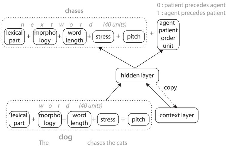
**Figure 4.** The architecture of the SC model. The figure refers to the English version and shows the presentation of the active sentence ‘The dog chases the cats’
